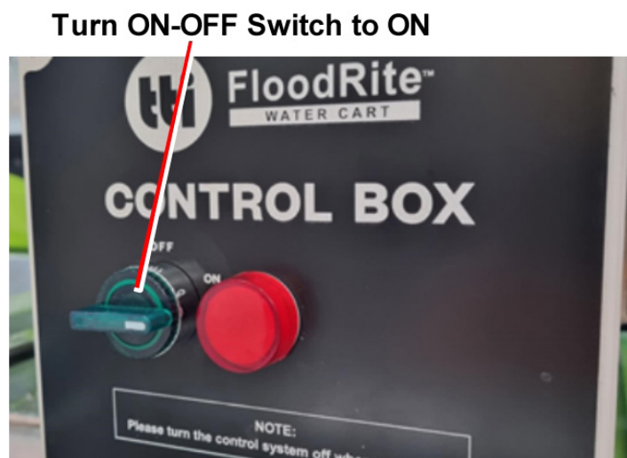
Figure 17 – Control Box ON-OFF Switch to ON
