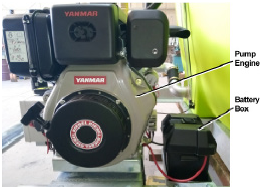
Figure 3 – Pump Engine and Battery (Diesel unit shown)
