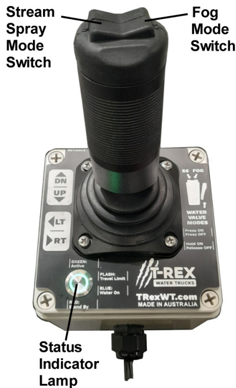
Figure 13 – Water Cannon Joystick Controller
