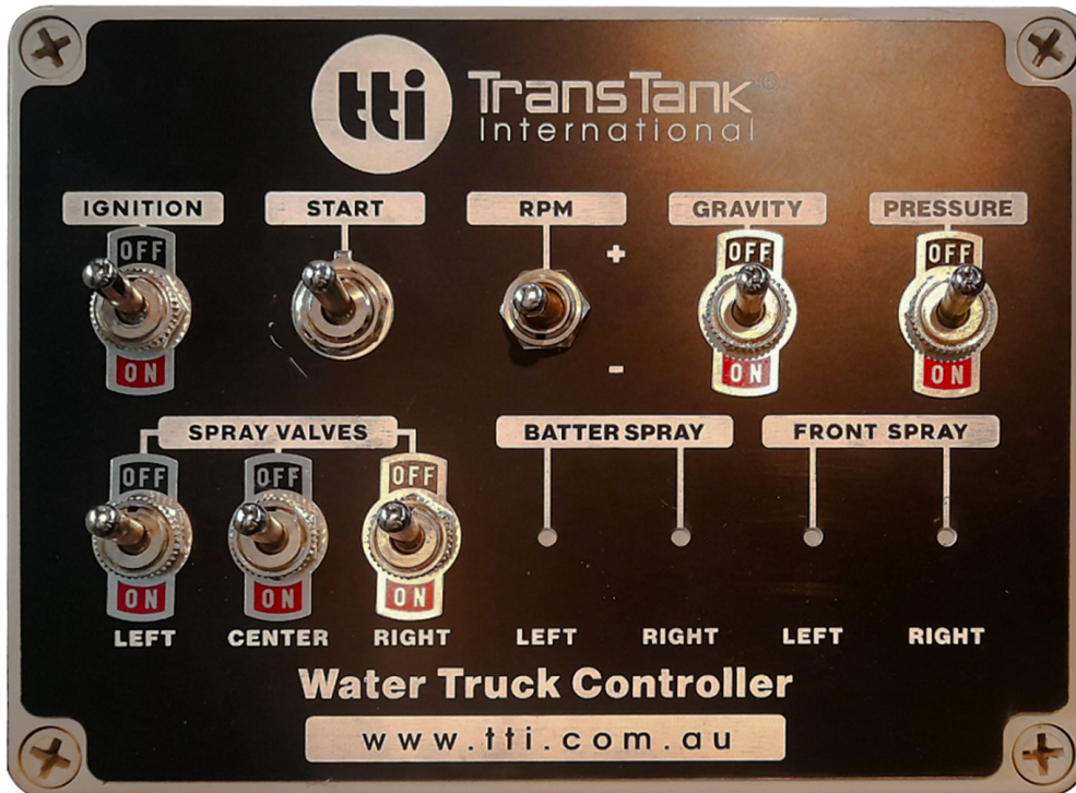
Figure 5 – In-cab Control Panel – Petrol/Diesel Pump Unit (typical)
