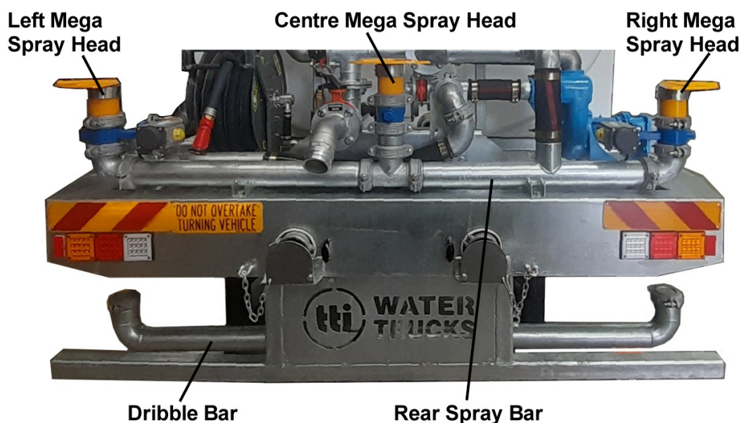
Figure 9 – Rear Spray Bar and Dribble Bar
