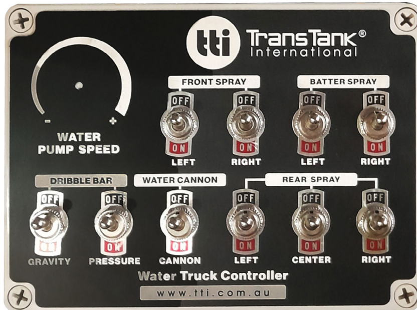
Figure 3 – In-cab Control Panel – Hydraulic Pump Unit
