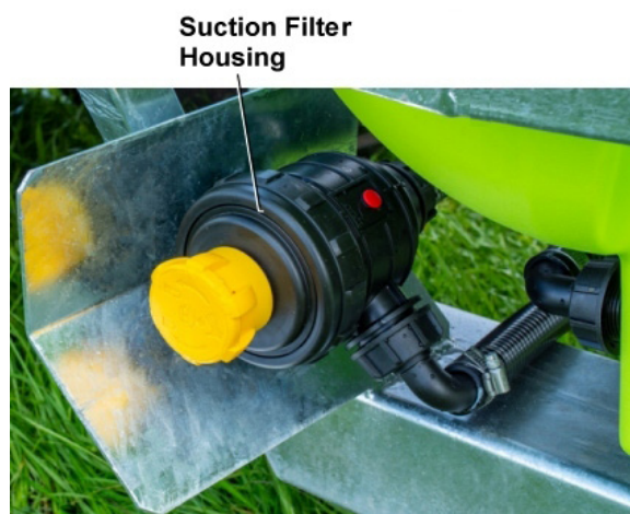
Figure 11 – Suction Filter (typical)
