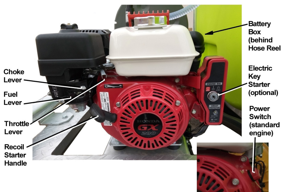
Figure 6 – Petrol Engine Start-up Procedure
