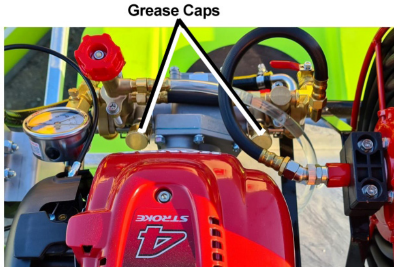
Figure 11 – Grease Caps Maintenance
