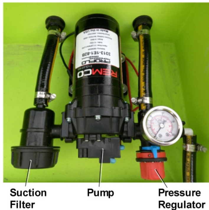
Figure 11 – Electric Pump's Suction Filter
