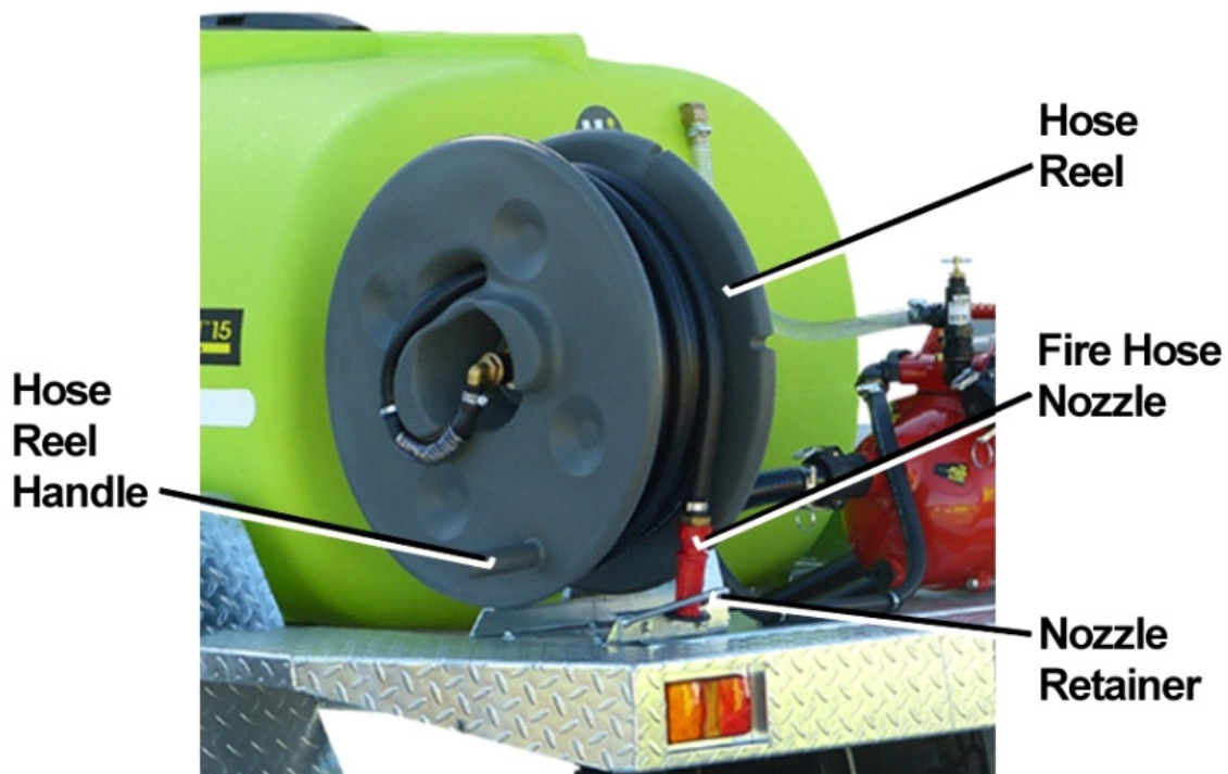
Figure 6 – Fire Hose Reel
