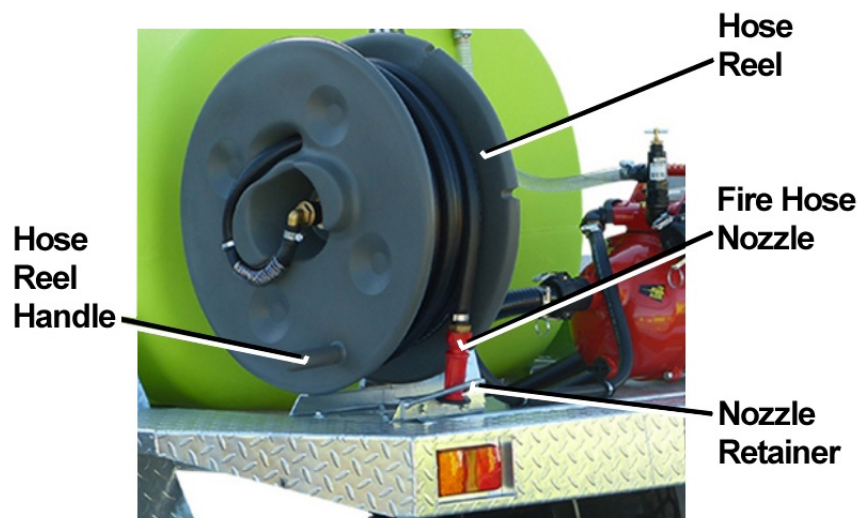
Figure 5 - Fire Hose Reel
