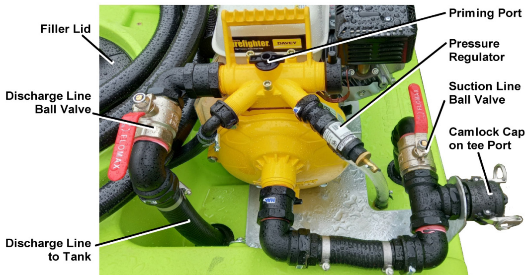
Figure 2 – Tank Filling Operation
