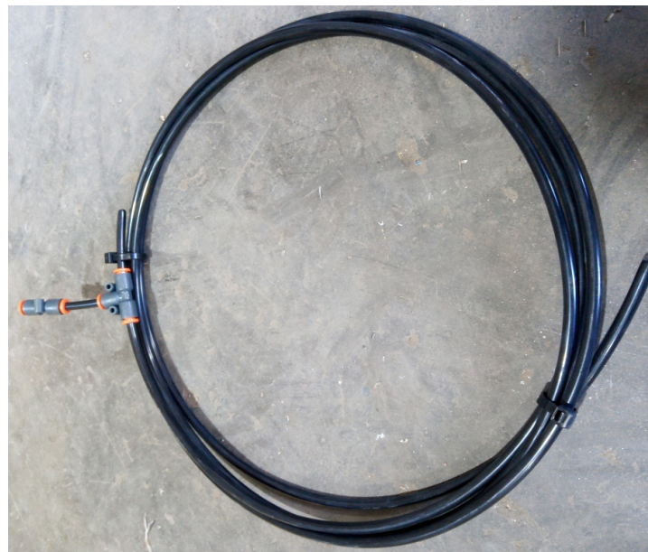
Figure 2 – Pneumatic Hose and Tee Piece
