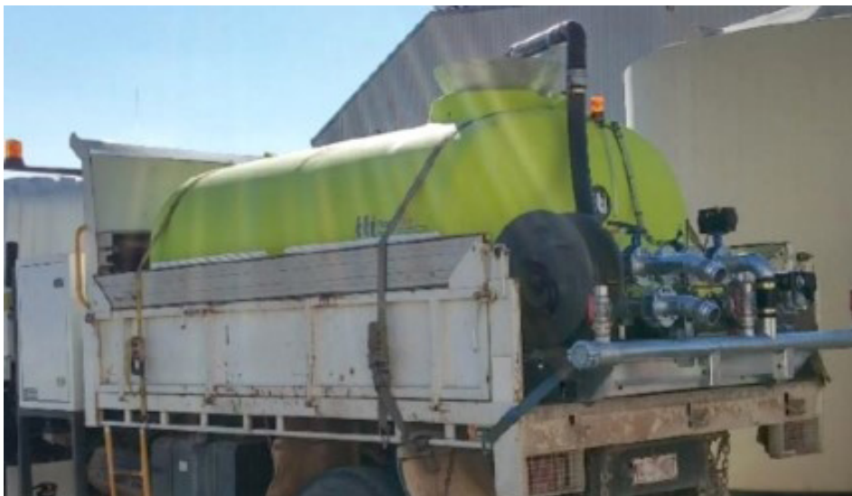
Figure 15 – Over Tank Strap Option (Typical)
