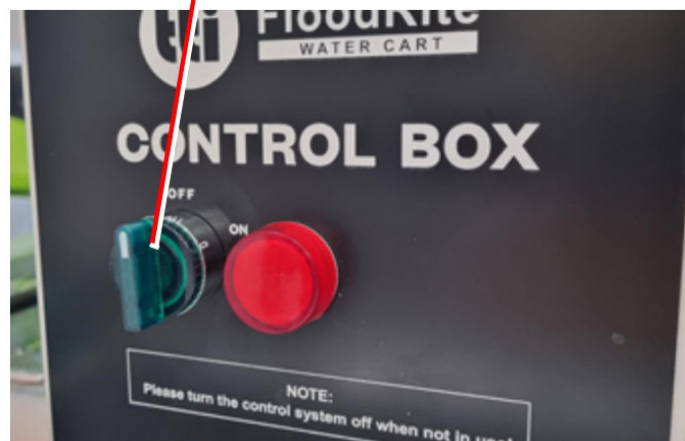
Figure 23 – Control Box ON-OFF Switch to OFF
