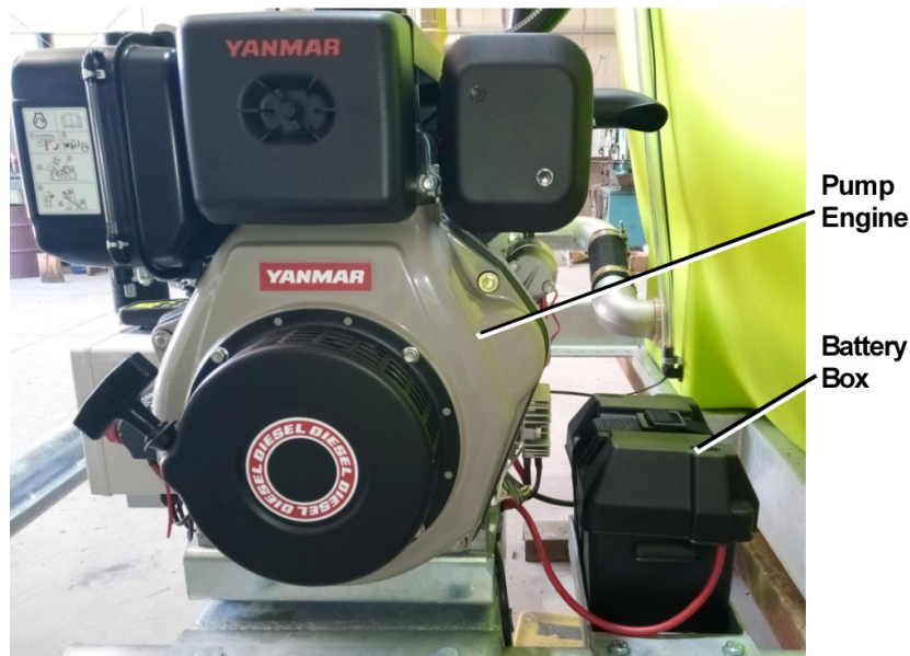
Figure 3 – Pump Engine and Battery (Diesel unit shown)
